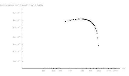
**EPU-1** - Circularly polarized first harmonic range includes 600-900 eV at high brightness (for magnetic studies).
