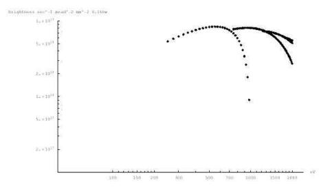
**EPU-2** - Linearly polarized first, third, fifth and seventh harmonic range. This is for E-vector in vertical orientation where the 10 mm internal vacuum tank size limits the lower energy achievable.
