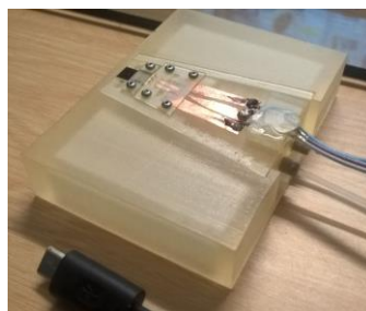
Figure 4.11 A completely assembled flow cell, ready to mount.
