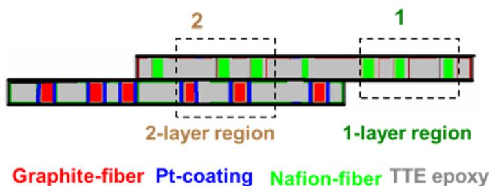
**Figure 3.2** Cartoon of structure of model sample used to evaluate the ability of STXM tomography to measure 3D distributions and ptychographic to measure non-crystalline soft matter with improved spatial resolution. The dashed boxes indicate the types of areas measured for the data presented in chapter 5
