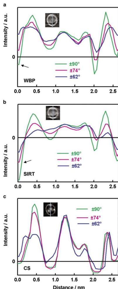
**Figure 10.** Line intensity profiles through selected  $xz$  planes from (a) weighted back-projection (WBP), (b) simultaneous iterative reconstruction technique (SIRT), and (c) compressed sensing total variation (CS-TV) reconstructions corresponding to the three tilt angle ranges indicated in Figure 9. The insets show the location of the selected lines.
