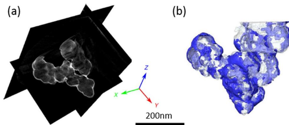
**Figure 2.2** (a) Three representative orthoslices of the reconstruction of STEM tomography of a PEMFC cathode; (b) 3D-rendered volume: the blue and grey regions correspond to the  $\text{Cs}^+$ -stained ionomer and to the carbon support, respectively (Lopez-Haro et al. 2014) (reproduced with permission from Springer Nature)
