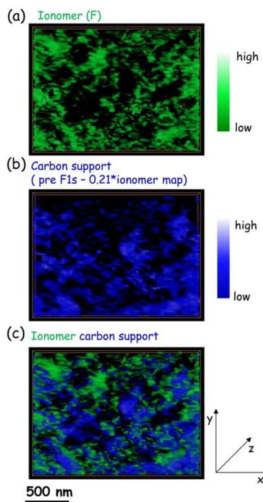
**Figure 7.** 4D imaging of the fuel cell cathode CL. Volume renderings of the 3D chemical structure of the cathode derived from a CS tomographic reconstruction of two-energy F 1s spectro-ptychotomography data. (a) Ionomer. (b) Carbon support. Threshold values for these renderings are 0.0023 for Ionomer and 0.0031 for carbon support. (c) Color composite (Ionomer in green, carbon support in blue) (ALS, 5.3.2.1).
