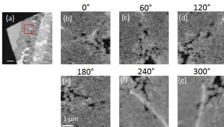
**Figure. A.3** (a) Laminography measurement region in red box, (b-g) 2D laminography carbon support maps at  $0^\circ$ ,  $60^\circ$ ,  $120^\circ$ ,  $180^\circ$ ,  $240^\circ$ ,  $300^\circ$  from the cathode region of a PEMFC.
