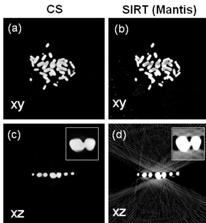
**Fig. S-3:** CS (left) and SIRT (right) electron tomography reconstructions of a Au nanoparticle sample using all 67 acquired projections. Selected slices through the  $xy$  plane of (a) CS, (b) SIRT and  $xz$  plane of (c) CS, (d) SIRT. The insets highlight the particles near the center of the volume.
