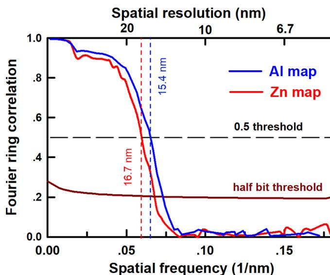
**Figure 7.8** Spatial resolution estimated from Fourier Ring Correlation (FRC) of the ZnO and Al<sub>2</sub>O<sub>3</sub> ptychography maps (Figs. 5c and 5d). (**sample B**).
