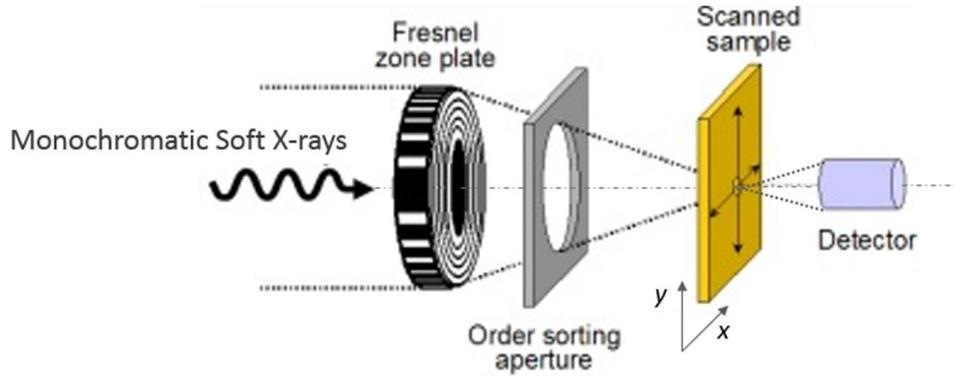
**Figure 2.8** Schematic diagram of STXM.
