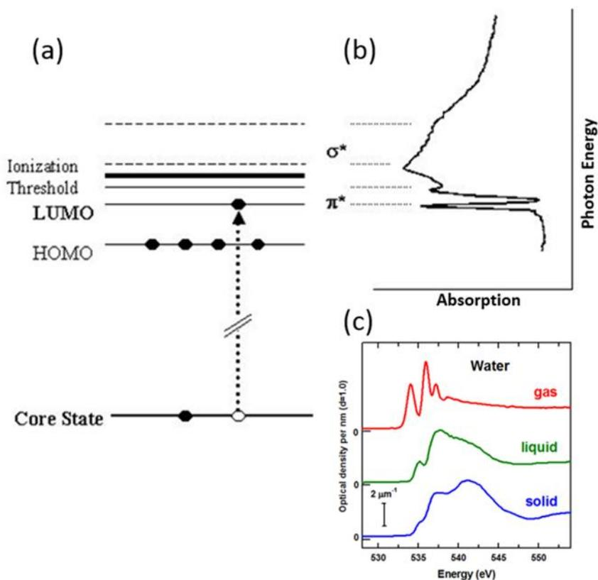
**Figure 2.7** (a) The near edge x-ray absorption fine structure (NEXAFS) arises from electronic transitions of an inner shell electron to energy levels (orbitals in molecules, bands in solids), (b) typical spectrum, (c) O1s spectra of gas, liquid and solid water.
