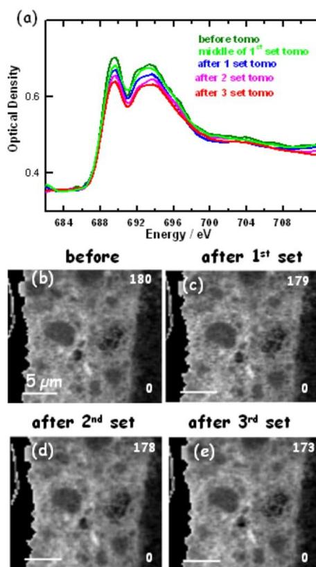
**Fig. S-7 (a)** F 1s spectra of PFSA (in cathode) measured at the indicated stages of 3 set spectro-tomography of sample MEA 11-GDE, tomography measurement **code G**. (b-e) 2D maps of the ionomer generated by a fit to the F 1s stacks: (b) before tomography, (c) after the 1<sup>st</sup> set, (d) after the 2<sup>nd</sup> set, (e) after the 3<sup>rd</sup> set. The numbers on the right side of each ionomer map are the gray scale limits in nm. (measured at CLS a-STXM, 10ID1)
