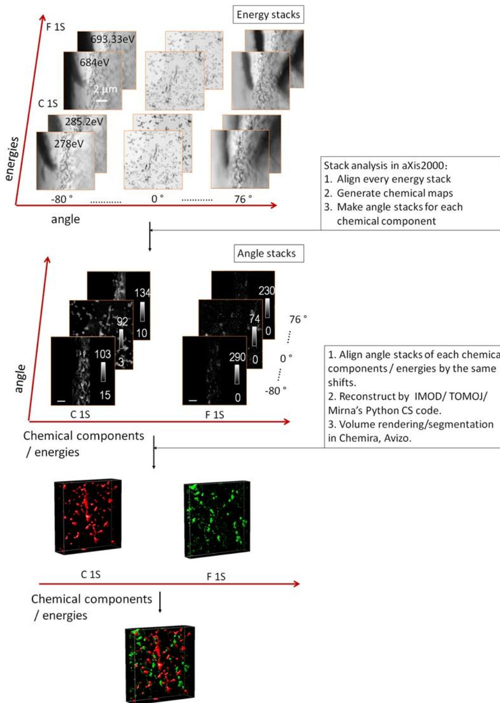
**Figure 3.9** STXM tomography data acquisition and analysis workflow
