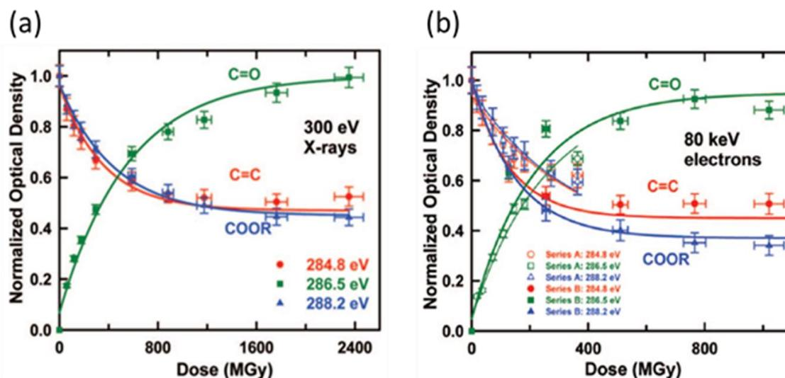
**Figure 2.11** Plots of the normalized optical density as a function of radiation dose for PET damaged at 284.8, 286.5, and 288.2 eV by exposure to (a) 300 eV X-rays; (b) 80 keV electrons (Wang *et al.*, 2009b) (reproduced with permission from American Chemical Society)
