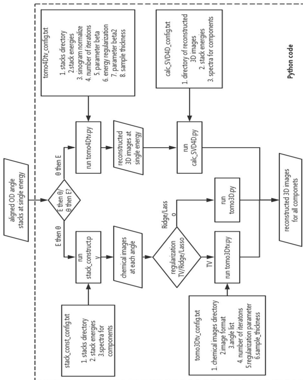
**Figure 3.11** Flow diagram of 4D data analysis process using Mantis python code
