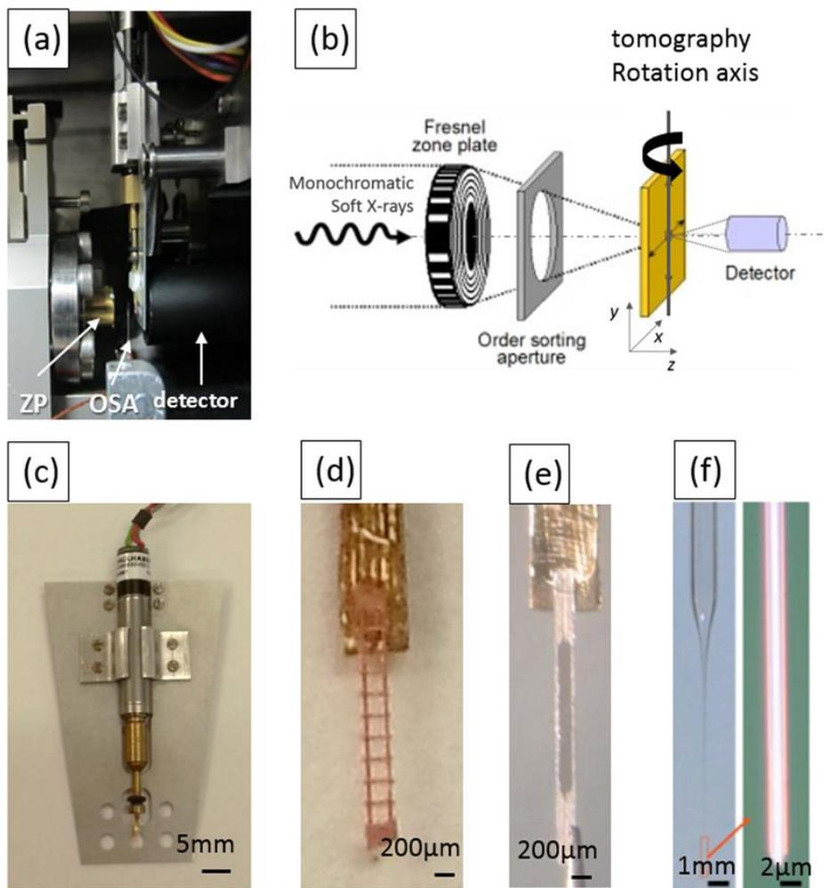
**Figure 3.5** (a) The STXM tomography stage mounted in ALS STXM 5.3.2.2; (b) schematic diagram of STXM tomography; (c) STXM tomography stage is composed of a stepper motor attached to a STXM sample plate. The sample is glued to the tip of a 0.8 mm diameter brass sample pin which is held in a chuck (taken from a mechanical pencil) attached to the motor shaft. STXM tomography samples: (d) TEM grid strip; (e) Luxel wet sample pin; (f) pulled glass capillary.
