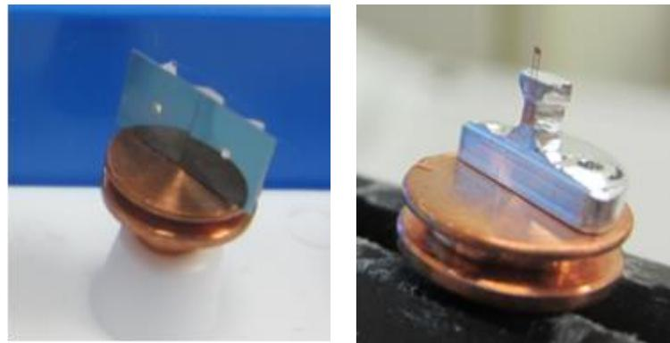
**Figure 3.18** Ptychography sample stage. (left) 2 SiN<sub>x</sub> windows or 2 TEM grids can be mounted. (right) grid strip mounted for tomography.
