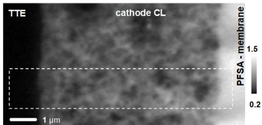
**Figure S-2.** STXM optical density image at 694 eV of the cathode region of a PEMFC membrane electrode assembly (MEA), recorded using a zone plate with 60 nm outer zone width. (ALS, 11.0.2)
