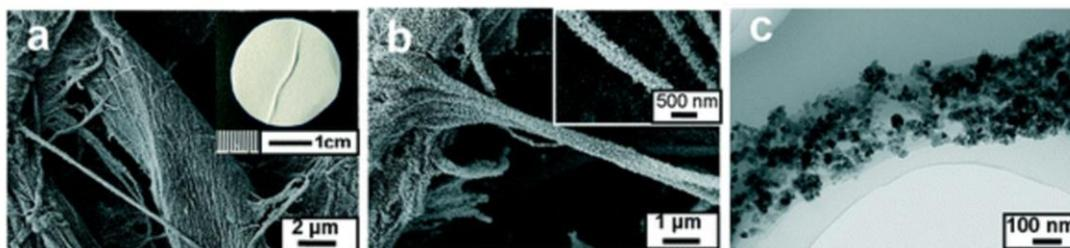
**Figure 8.5** (a) Low-magnification FE-SEM image; (b) high-magnification FE-SEM image; (c) TEM of an individual anatase-titania–cellulose composite nanofibre isolated from the assembly (Luo et al. 2014) (Reproduced with permission from Royal Society of Chemistry)
