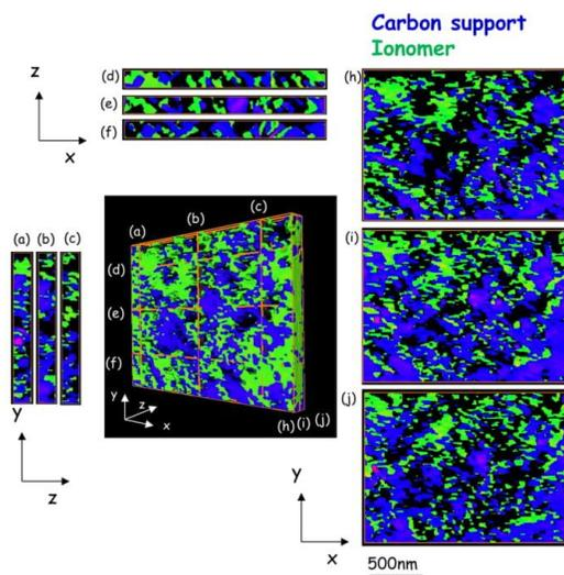
**Figure 8.** Multiple slices from the 3D rendered volume of the two components derived from F 1s spectro-ptycho-tomography. (a–c) In zy plane, (d–f) in xz plane, and (h–j) in xy plane. (g) indicates the position of each slice in the volume image. Threshold values for the slices are 0.0031 for the ionomer and 0.0023 for the carbon support. See Supporting Information for a movie with a detailed rendering and display of this 4D reconstruction (ALS, 5.3.2.1).
