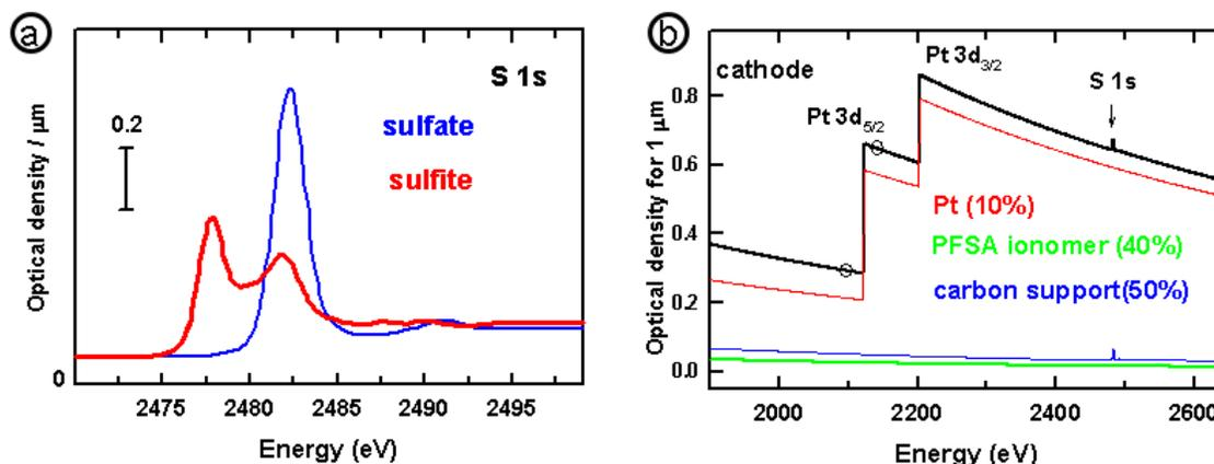
**Fig. 8.1** Evaluation of S 1s STXM of cathodes. (a) S 1s spectra of sulfate and sulfite species (Hay et al 2004). (b) Simulation of Pt 3d and S 1s region of the X-ray absorption spectra of a cathode, consisting of 10 % Pt (red), 50 % carbon support (blue), and 40 % PFSA ionomer (green).
