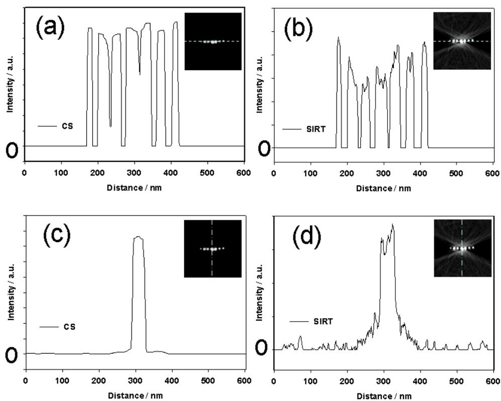
**Fig. S-4:** Line intensity profiles through  $xz$  plane from the (a),(c) CS and (b),(d) SIRT reconstructions shown in Fig. S-3
