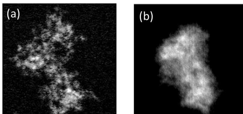
**Figure A.10** (a) 2D images of the TiO<sub>2</sub> / Al<sub>2</sub>O<sub>3</sub> aerogel sample at 0°; (b) 0° view of the 3D reconstructed volume
