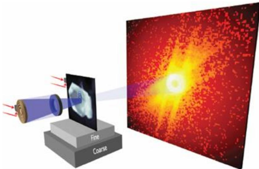
**Figure 2.4** Schematic of ptychography. A 60 nm coherent soft X-ray spot, focused by zone plate, is scanned over the sample in 40 nm increments. (Shapiro *et al.*, 2014) (reproduced with permission from Springer Nature)
