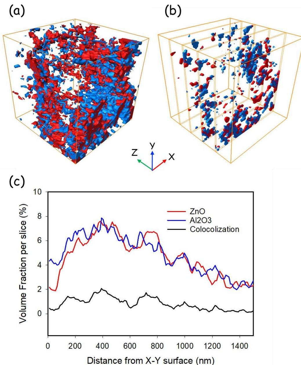
**Figure 7.12** (a) Surface rendering of  $(1.5 \mu\text{m})^3$  center cube of the reconstructed ptychographic spectro tomography data (**sample B**). (b) single slices at 0.3  $\mu\text{m}$ , 0.6  $\mu\text{m}$ , 0.9  $\mu\text{m}$  and 1.2  $\mu\text{m}$  depth of the cube. c) plot of the volume fraction per slice, as a function of depth from the xy surface.
