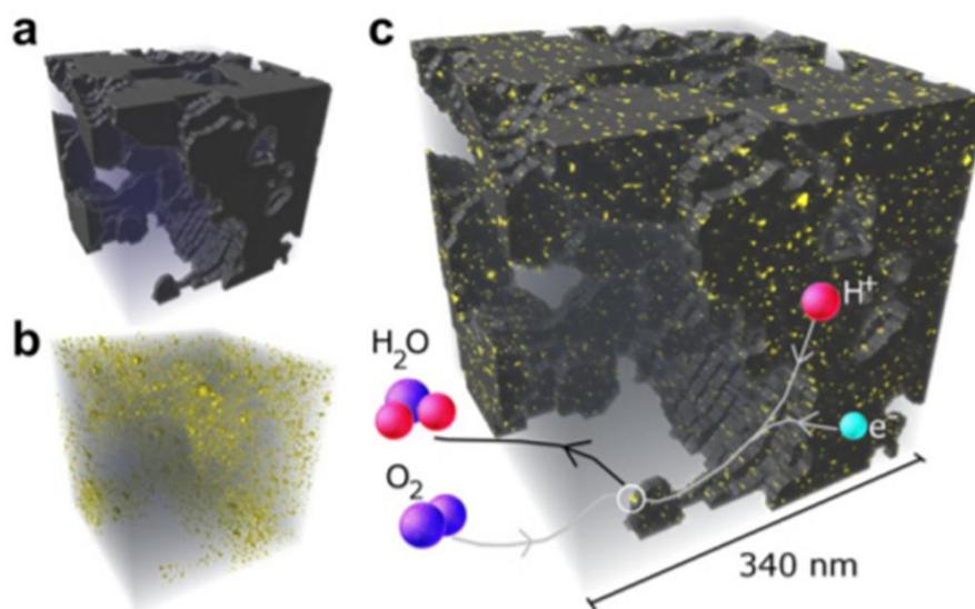
**Figure 1.7** (a) A cube of 340 nm side length of the SEMt reconstruction. (b) The reconstructed Pt volume information in the same spatial area as the SEMt reconstruction. (c) The superposition of (a) and (b) and visualizes the location of Pt catalyst particle volume and surface information within the porous carbon matrix. (Thiele et al. 2013)(reproduced with permission from Elsevier)
