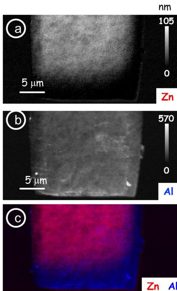
**Figure 7.2** STXM 2D chemical maps at 0° tilt angle of a ZnO/Al<sub>2</sub>O<sub>3</sub> aerogel (**sample A**).
