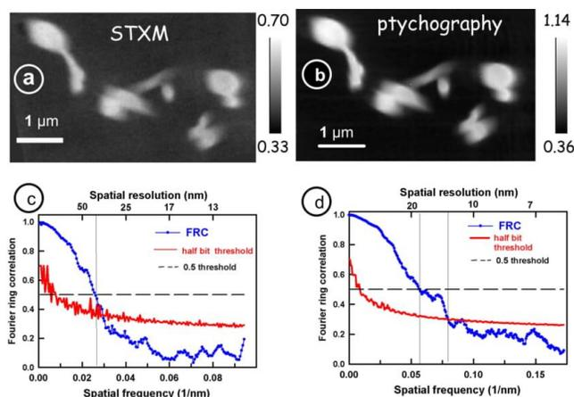
**Figure 2.** Images of the single layer region of the bilayer model sample (see Figure 1). (a) STXM OD image at 694 eV recorded with 1 ms/pixel sampling, using a ZP with 25 nm outer zone width (recorded after ptychography) (CLS 10ID1). (b) Ptychography absorption image at 694 eV of the same area. (c) FRC analysis of the spatial resolution for the STXM image of (a). (d) FRC analysis for the ptychography image of (b) (ALS 5.3.2.1).
