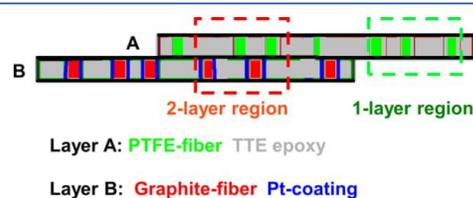
**Figure 1.** Cartoon of structure of the model sample used to evaluate the resolution improvement when using soft X-ray ptychography to measure noncrystalline soft matter. The dashed boxes indicate the type of areas measured for the data in Figure 2 (1-layer) and Figure 4 (2-layer).
