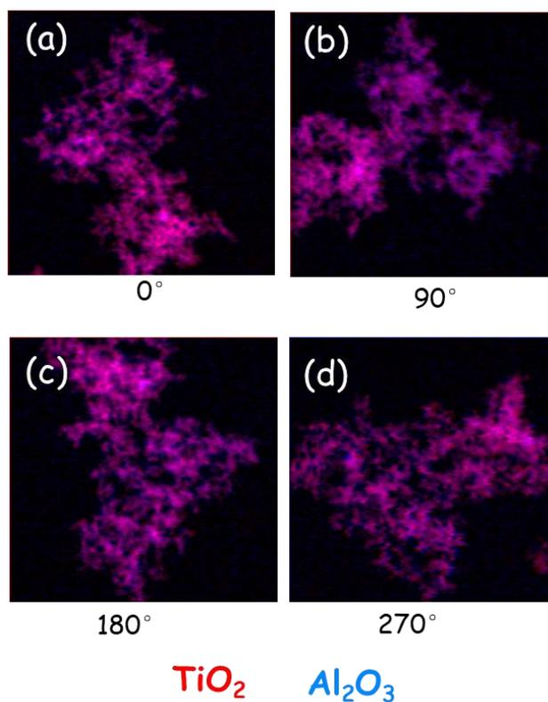
**Figure A.7** Chemical maps of TiO<sub>2</sub> (red) Al<sub>2</sub>O<sub>3</sub> (blue) at rotation position (a) 0°, (b) 90°, (c) 180°, (d) 270°
