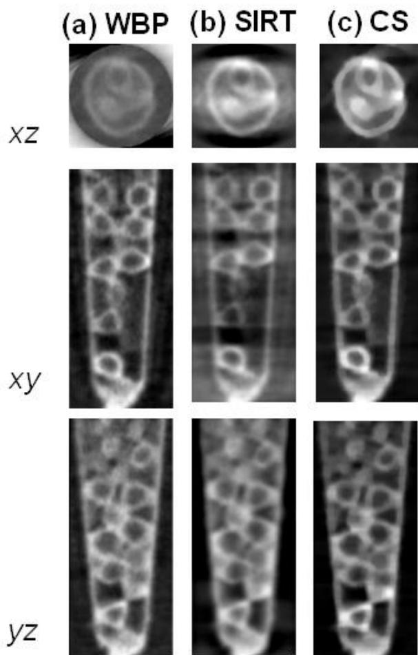
**Fig. S-5:** Tomographic reconstructions of the STXM images at 290 eV for  $\pm 90^\circ$  tilt angle ranges using (a) WBP, (b) SIRT and (c) CS-TV. Slices through the  $xz$  (top),  $xy$  (middle) and  $yz$  (bottom) planes are shown for each reconstruction.
