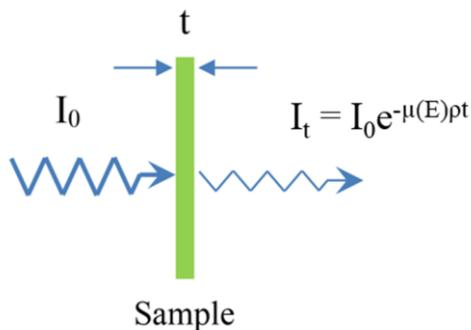
**Figure 2.9** The transmitted photon intensity  $I_t$  is related to the incident photon intensity  $I_0$ , mass absorption coefficient  $\mu$ , the sample density  $\rho$ , and the sample thickness  $t$ .
