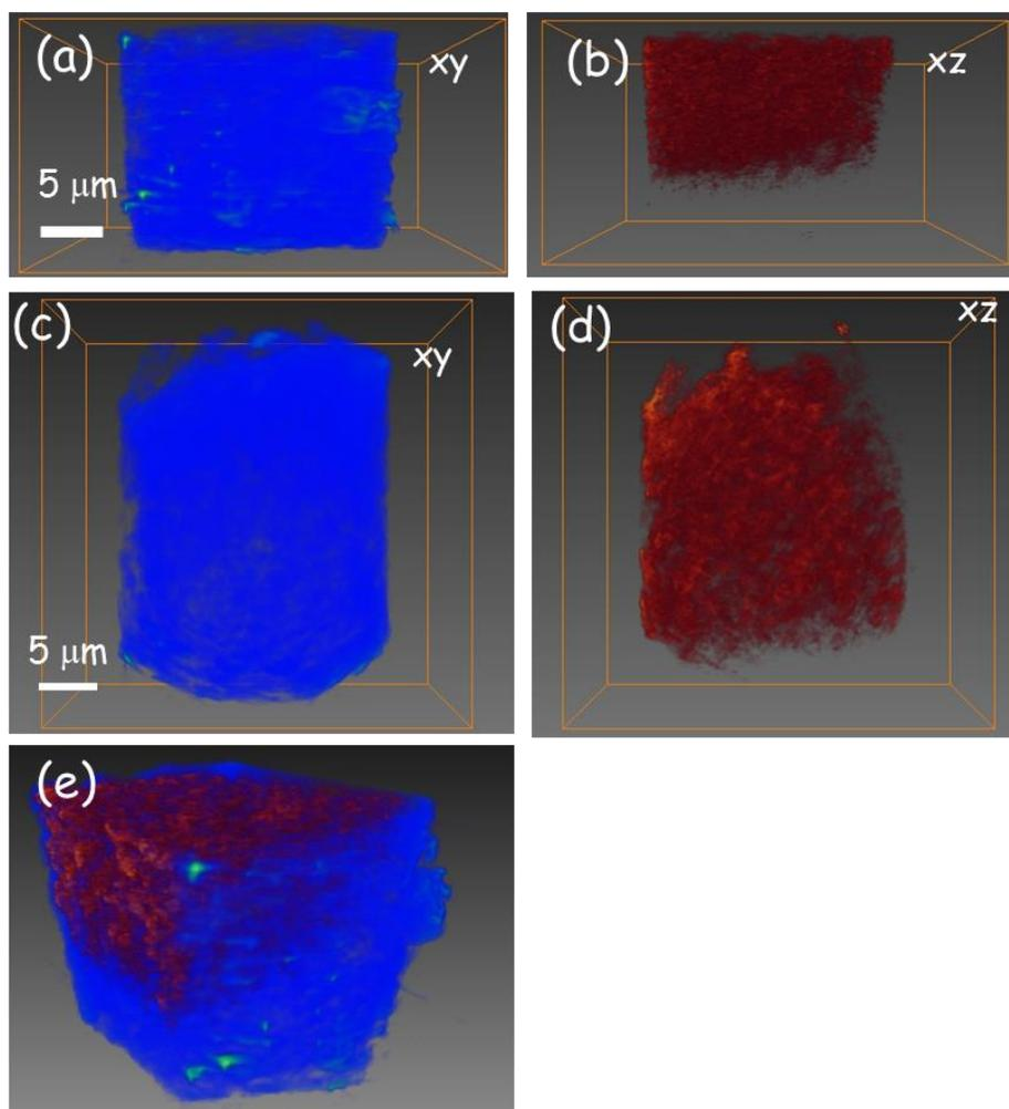
**Figure 7.3** STXM spectro-tomography derived, 3D volume rendering of Al<sub>2</sub>O<sub>3</sub> (blue) and ZnO (red) in the ZnO/Al<sub>2</sub>O<sub>3</sub> aerogel FIB **sample A**. (a, b) xy views. (c,d) xz views. (z is direction of X-ray beam). (e) 4D image, a color coded composite of the two components with Al<sub>2</sub>O<sub>3</sub> in blue and ZnO in red. Otsu threshold for ZnO is 0.0004, for Al<sub>2</sub>O<sub>3</sub> is 0.0001.
