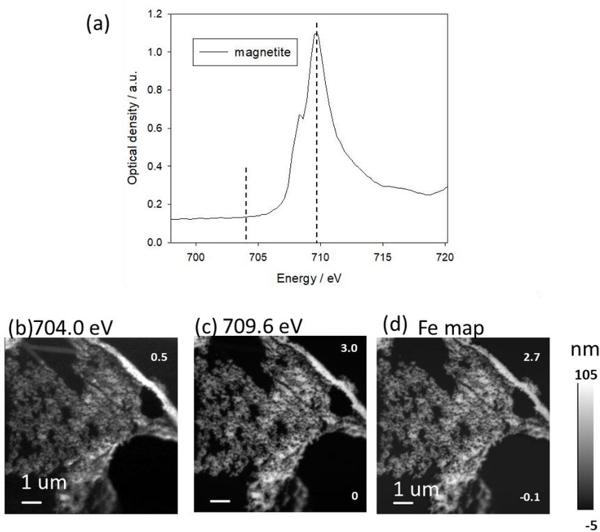
**Figure A.1** (a) Fe 2p<sub>3/2</sub> spectrum of magnetite; (b) 2D images at 704 eV; (c) 2D images at 709.6 eV; (d) Fe map generated by OD<sub>709.6</sub>-OD<sub>704</sub>
