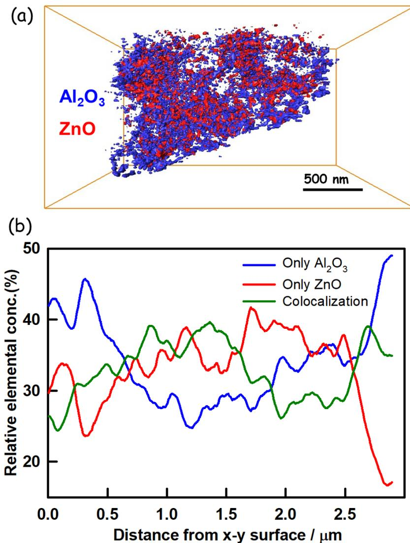
**Figure 7.10** a) Surface rendered color coded composite of the 3D distributions of ZnO and Al<sub>2</sub>O<sub>3</sub> from ptychography of ZnO/Al<sub>2</sub>O<sub>3</sub> aerogel (**sample B**). (b) Volume fraction of the two components and their co-localized amounts in the solid portion of xy slices through the
