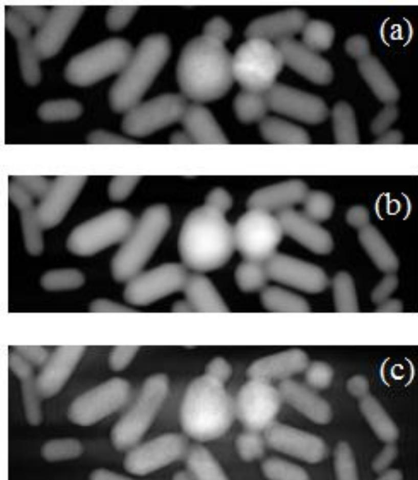
**Figure S-2** Comparison of (a) original image from tilt series at  $0^\circ$ . (b) 2D projection at  $0^\circ$  generated from CS reconstruction. (c) 2D projection at  $0^\circ$  generated from the SIRT reconstruction. All 67 tilt angles were used.
