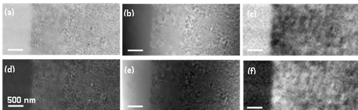
**Figure 3.21** Ptychographic reconstructed data measured at 720 eV of a region consisting of the membrane and part of the cathode of a PEMFC. (a) modulus (amplitude) image, (b) phase image, (c) stxm image, (d) ( $I_0$ -corrected amplitude) absorption and (e)  $I_0$ -corrected phase image (f)  $I_0$ -corrected stxm image (5.3.2.1 run of May 2016, data set 2016-05-20-021)
