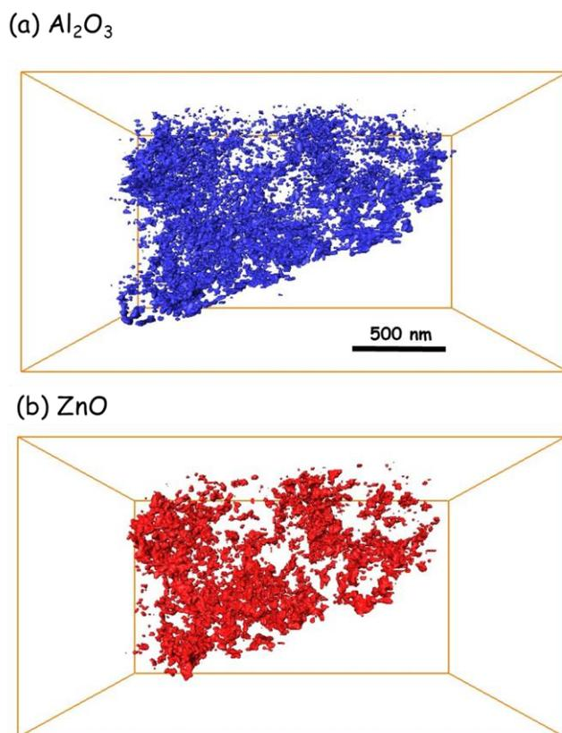
**Figure 7.7** 3D surface rendering of ZnO and Al<sub>2</sub>O<sub>3</sub> from ptychography of ZnO/Al<sub>2</sub>O<sub>3</sub> aerogel (**sample B**). View at 0° of (a) Al<sub>2</sub>O<sub>3</sub> (blue), derived from the signal at 1010 eV minus 17 % of the ZnO signal. (b) ZnO (red) (OD(1026.8 eV) – OD(1010 eV)). The voxel size is (5.6\*5.6\*5.6) nm<sup>3</sup>. The Otsu thresholds used were 0.0018 for the Al<sub>2</sub>O<sub>3</sub> signal and 0.0026 for the ZnO signal.
