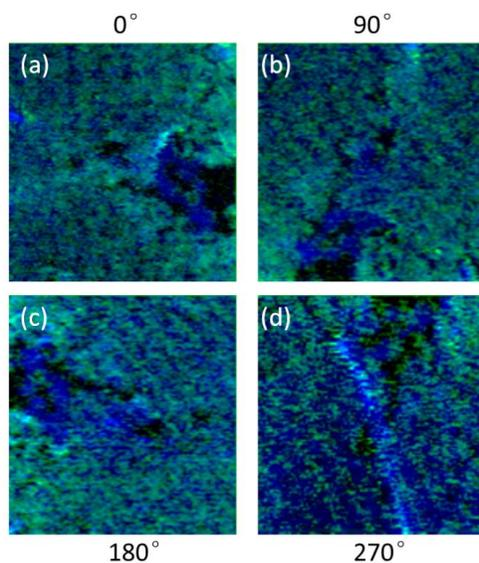
**Figure A.4** Chemical maps of carbon support (blue) and ionomer (green) at (a)  $0^\circ$ , (b)  $90^\circ$ , (c)  $180^\circ$ , (d)  $270^\circ$
