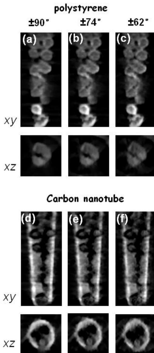
**Fig. S-6:** Tomographic reconstructions using SIRT with a non-negativity constraint of the polystyrene (PS) (a,b,c) and carbon nanotube component s(d,e,f) for three different tilt angle ranges (a,d)  $\pm 90^\circ$ , (b,e)  $\pm 74^\circ$ , and (c,f)  $\pm 62^\circ$ . Slices through the  $xy$  (top) and  $xz$  (bottom) planes are shown for each reconstruction.
