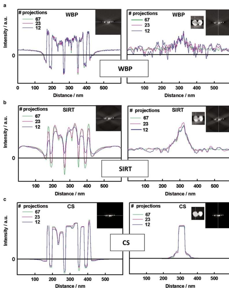
**Figure 3.** Line intensity profiles through  $xz$  planes for (a) weighted back-projection (WBP), (b) simultaneous iterative reconstruction technique (SIRT), and (c) compressed sensing (CS) tomographic reconstructions using 67, 23, and 12 projections as in Figure 2. The insets show the locations of the selected lines.
