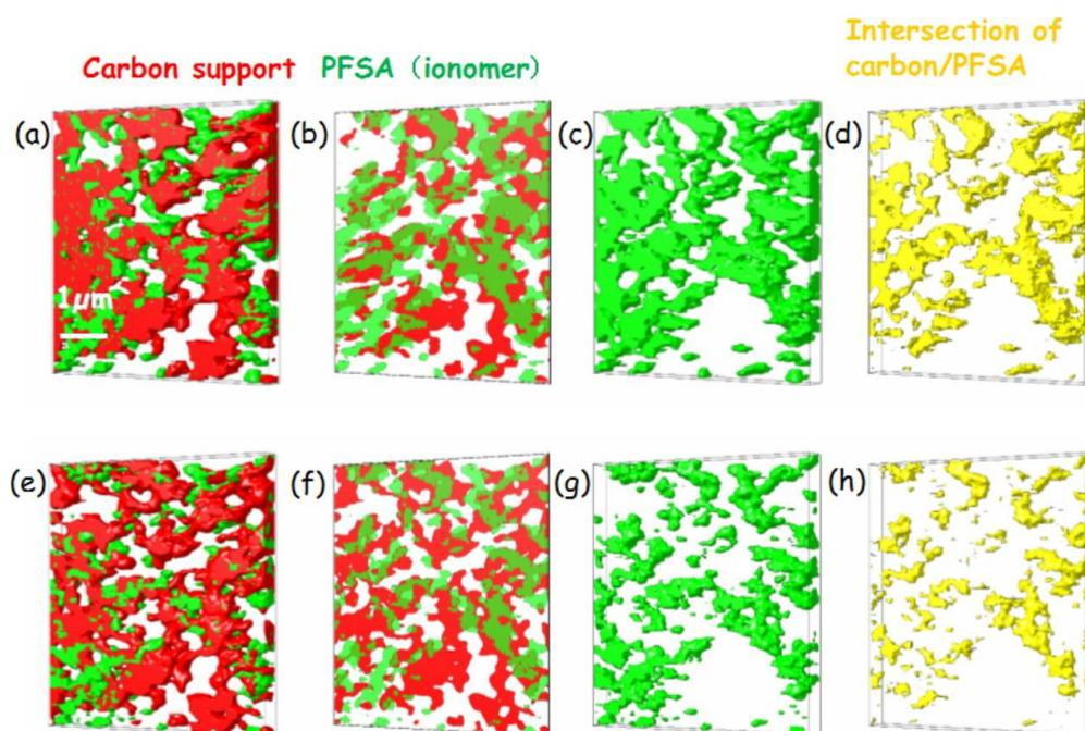
**Fig. S-6** 3D distributions viewed at a tilt of  $-30^\circ$  of carbon support (red) and ionomer in cathode (green) of sample MEA-A, **code E**, low dose cut at a nominal thickness of 100 nm. (a,b,c,d) are from set 1. (e,f,g,h) are from set 2. The yellow display in (d) and (h) is the intersection of the maps of the carbon support and ionomer. Otsu thresholds for set 1 (2) are 0.007 (0.005) for ionomer, and 0.0095 (0.0075) for carbon support. (measured at ALS1102, and CLS 10ID1).
