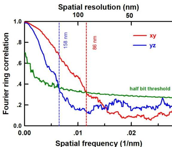
**Fig. S-10** Spatial resolution estimated from Fourier ring correlation (FRC) of a slice through the central x-y and y-z directions in the reconstructed tomography results for MEA-A in PS **code F**. (measured at ALS 11.0.2)
