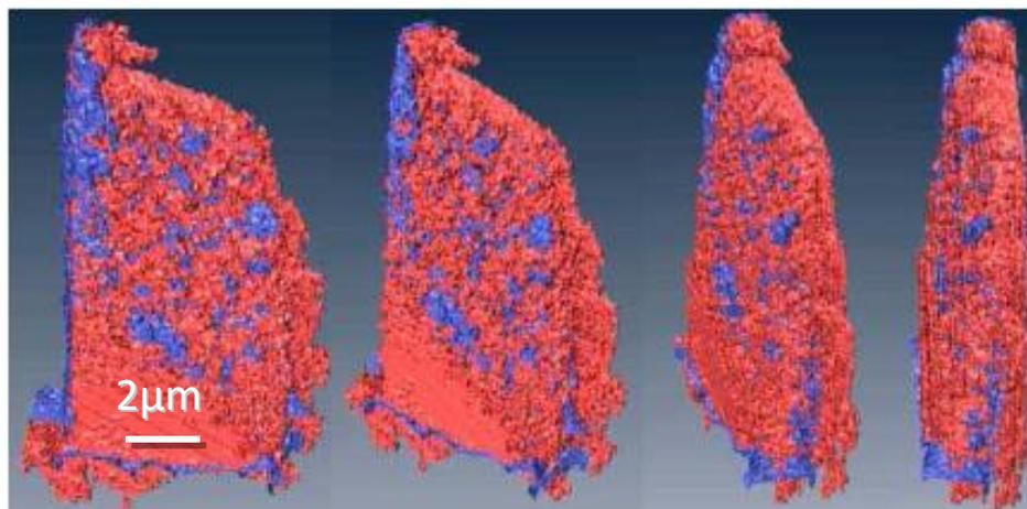
**Figure 2.3** 3D chemical maps in 0°, 30°, 60°, 90° degree projections extracted from reconstructed volume with different threshold. The red signal represents the carbon support ( $OD_{285}-OD_{278}$ ) and the blue one shows the ionomer ( $OD_{296} - (OD_{285}-OD_{278})$ ) (Berejnov et al. 2013). (reproduced with permission from ECS Transactions) 50(2): 361-368. Copyright 2013, The Electrochemical Society)
