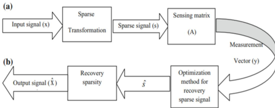
**Figure 2.13** Compressed sensing model.
