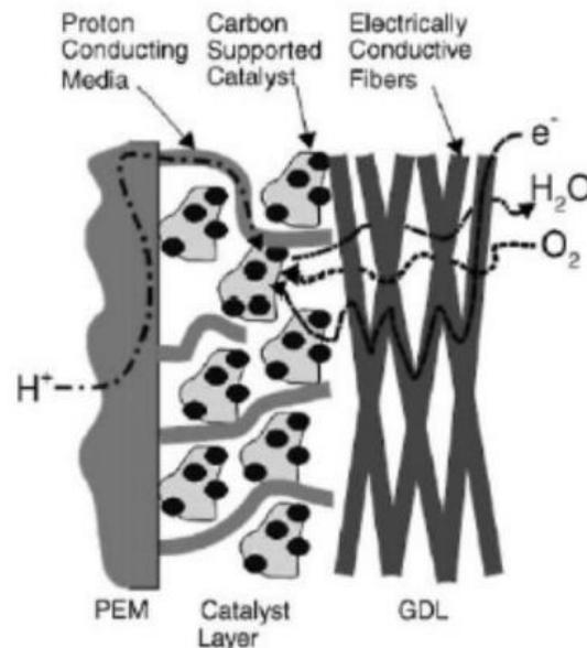
**Figure 1.6** Schematic diagram of PEMFC cathode catalyst (Litster and McLean 2004)
