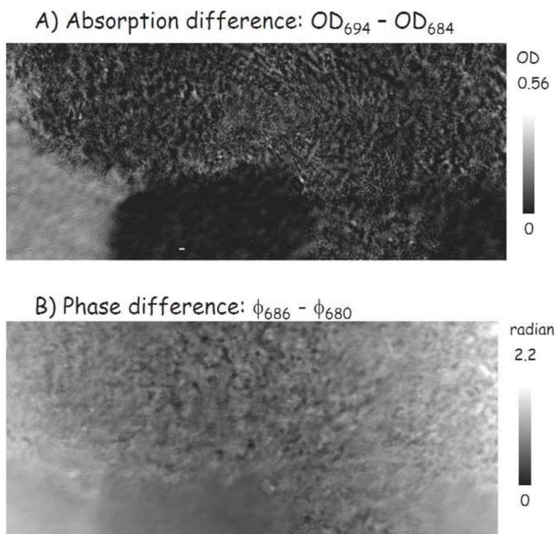
**Figure S-1 (a)** Ptychography absorption difference image ( $OD_{694} - OD_{684}$ ). **(b)** Phase difference image (phase(686 eV) – phase(680 eV)) derived from the same ptychography stack data set.
