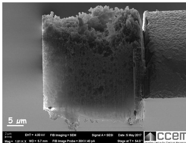
**Figure 3.3** Scanning electron microscope (SEM) image of FIB sample of ZnO/Al<sub>2</sub>O<sub>3</sub> aerogel sample
