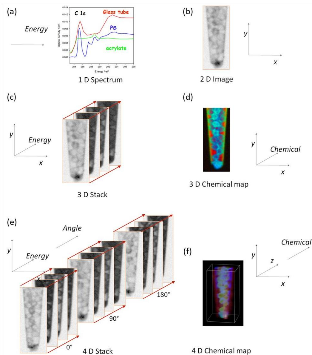
**Figure 1.1** Image of a sample consisting of polyacrylate-filled polystyrene microspheres in water inside a pulled glass capillary (a) 1D C 1s X-ray absorption spectra, (b) 2D image, (c) 3D stack, (d) 3D chemical map, (e) 4D stack, (f) 4D image. The 3D stacks (e) at each scan angle contained 23 energy images.
