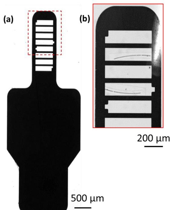
**Figure 3.23** Gatan ‘flyswatter’ sample grid. There are supplied bare and a layer of formvar was added prior to mounting microtomed MEA samples. (a) Full grid, (b) expand tip shown an MEA sample on formvar
