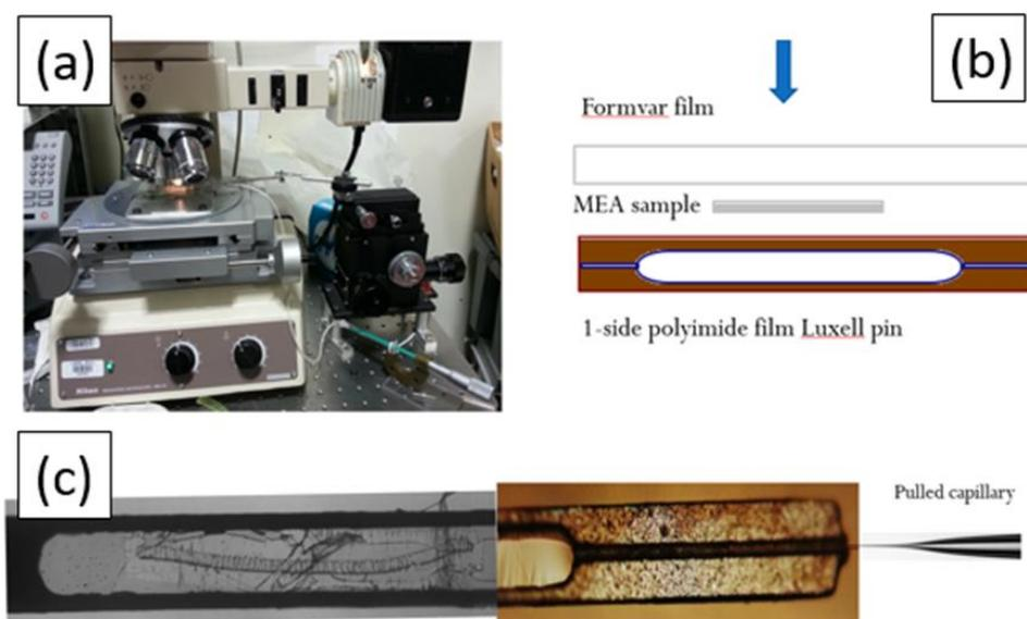
**Figure 3.6** (a) The setup for injecting water to make a Luxel tomo wet cell (ALS 11.0.2). A 1 mL syringe connected to a glass micropipette is used as a micro-injector. (b) MEA sample is mounted on the 1-side (bottom) polyimide film Luxel window, then a formvar film is added on top, which forms a closed window. (c) The tip of the glass capillary should stick into the channel of the Luxel pin to define the water path.
