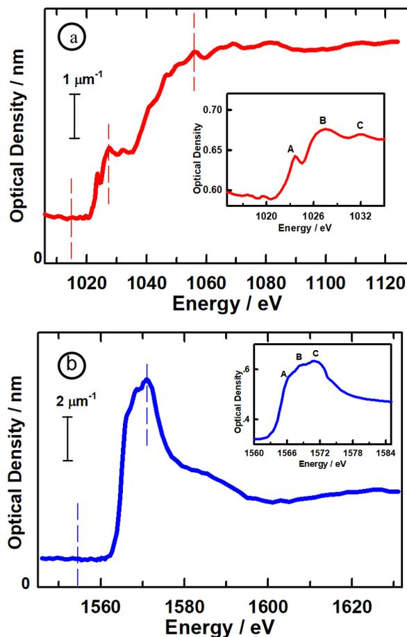
**Figure 7.1** (a) X-ray absorption spectra (XAS) of ZnO/Al<sub>2</sub>O<sub>3</sub> aerogel (**sample A**). (a) Zn L<sub>2,3</sub> edge, converted to optical density per nm (OD1). The inset shows an expanded view of the near edge L<sub>3</sub> region. (b) Al K edge, converted to optical density per nm (OD1). The inset shows an expanded view of the near edge.
