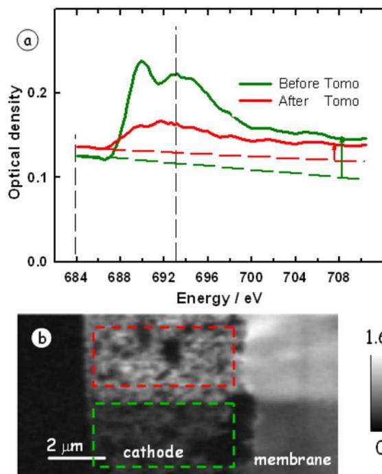
**Fig. S-3 (a)** Average F 1s spectra of PFSA in cathode of sample MEA-A, **code D** (table 2), before and after 3 set spectro-tomography. **(b)** Fluorine map derived from a F 1s stack (81 images from 678 to 730 eV) measured after 3-set F1s tomography. The rectangular frames indicate the regions of the cathode where the undamaged (green) and damaged (red) spectra were extracted. (measured at ALS 11.0.2)
