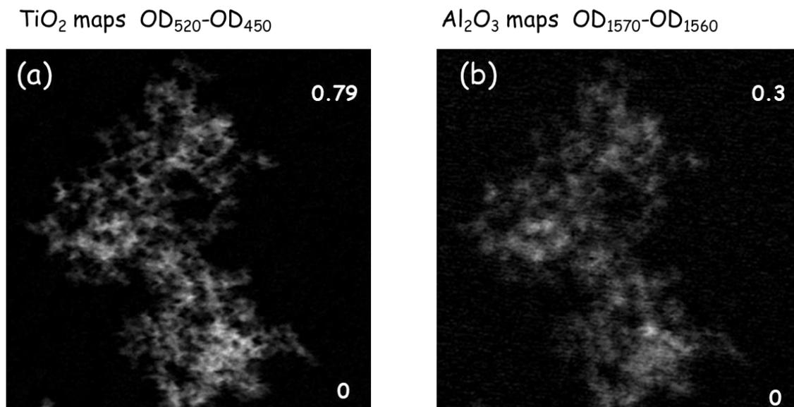
**Figure A.6** Chemical maps of (a) TiO<sub>2</sub> generated by OD<sub>520</sub>-OD<sub>450</sub> (b) Al<sub>2</sub>O<sub>3</sub> generated by OD<sub>1570</sub>-OD<sub>1560</sub>
