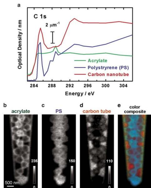
**Figure 8.** a: C 1s spectra of the components of a sample consisting of acrylate filled polystyrene microspheres inside a carbon nanopipette. Quantitative two-dimensional projection components maps (thicknesses in nm) of (b) acrylate, (c) polystyrene (PS) microsphere shell, and (d) the carbon nanotube pipette. e: Color-coded composite map showing acrylate in green, PS in blue, and the carbon nanotube pipette in red.
