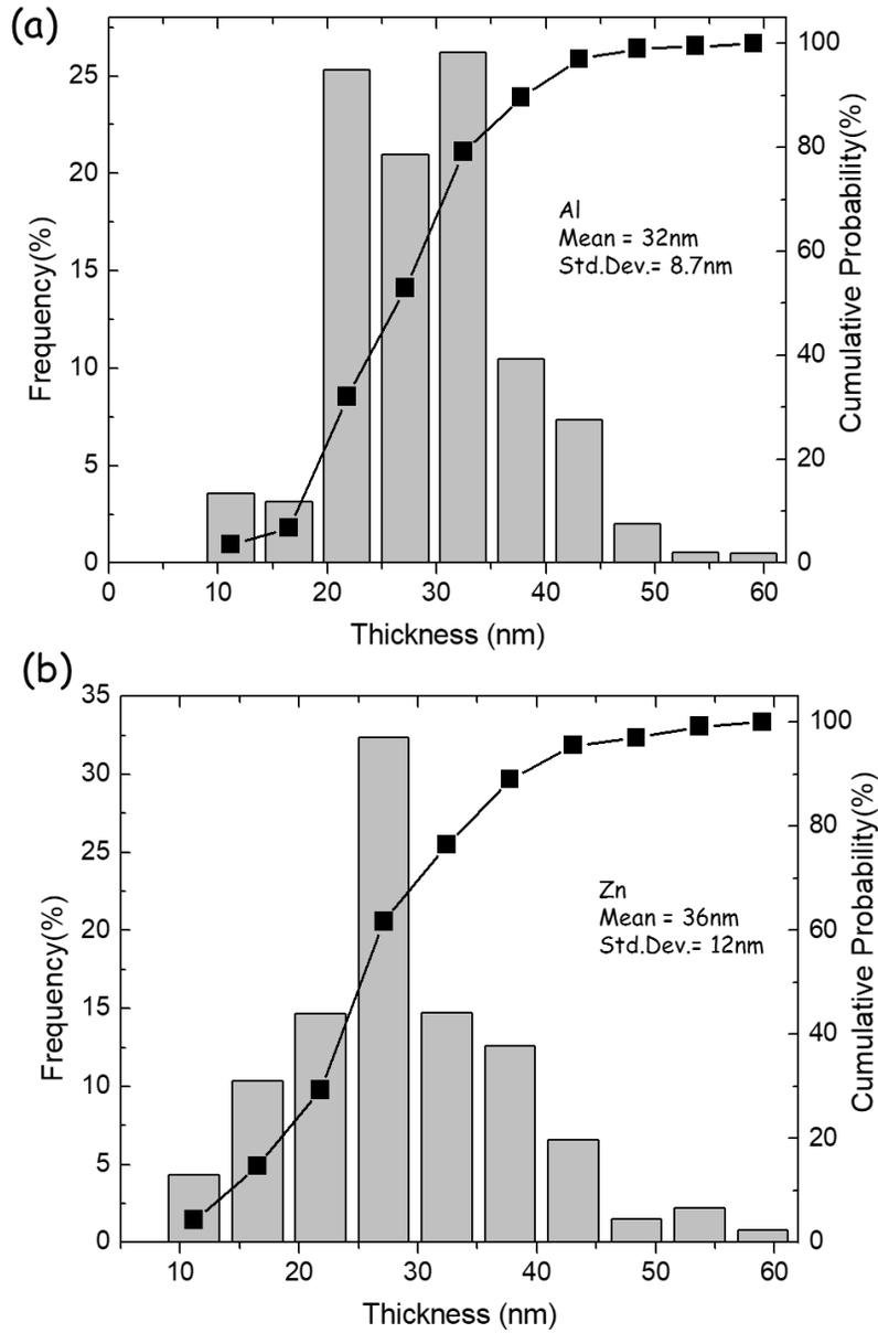
**Figure 7.9** Histogram of the thickness distribution of (a) Al<sub>2</sub>O<sub>3</sub> signal and (b) ZnO signal, in the aerogel sample measured by ptychography (**sample B**), derived using the ‘Bone J’ plugin in Image J. The square data points and curve are the cumulative probability of the thickness distributions.
