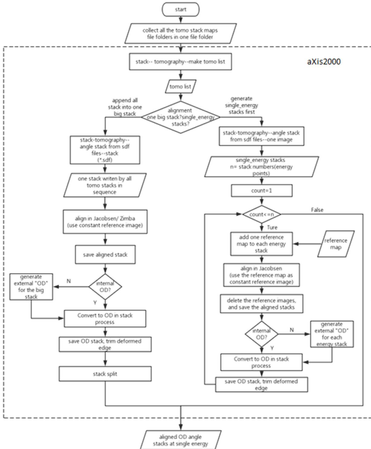
**Figure 3.10** Flow diagram of 4D data analysis process in aXis2000.
