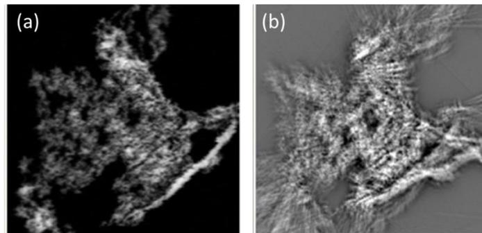
**Figure A.8** (a) 2D images of the magnetite at  $0^\circ$ ; (b)  $0^\circ$  view of the 3D reconstructed volume
