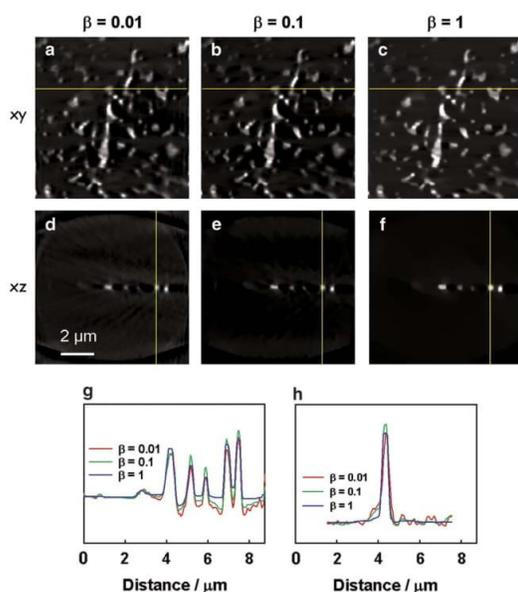
**Figure 7.** Effect of different choices of the  $\beta$  parameter for compressed sensing total variation (CS-TV) tomographic reconstructions. Slices through the  $xy$  (upper) and  $xz$  (middle) planes are shown for reconstructions using (a,d)  $\beta = 0.01$ , (b,e)  $\beta = 0.1$ , and (c,f)  $\beta = 1$ . g: Line intensity profiles through the indicated line on the  $xy$  slices. h: Line intensity profiles through the indicated line on the  $xz$  slices.
