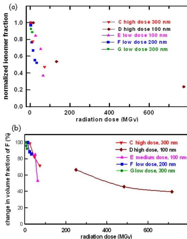
**Fig. S-9** (a) Fluorine loss as a function of dose caused by radiation damage in tomography for data sets **C - G**. The fluorine loss was normalized to the F 1s signal from the undamaged sample for each measurement. (b) Change in the volume fraction of ionomer between different sets as a function of radiation dose for data sets **C - G**. (numerical data is presented in table 3).
