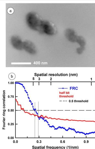
**Figure 3.** (a) TEM image of a fresh area of the PTFE single layer of the bilayer sample (bright field, 100 keV). (b) FRC analysis of spatial resolution of the TEM image, verifying that the edges of the PTFE fibers are sharp at a spatial scale significantly lower than that measured by ptychography.
