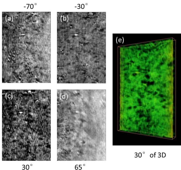
**Figure 8.2** 2D chemical maps of PFSA of an MEA sample under cryo conditions ( $-181^{\circ}\text{C}$ ) at different tilted angles, derived from images measured at 684eV and 694 eV. (a)  $-70^{\circ}$ , (b)  $-30^{\circ}$ , (c)  $30^{\circ}$ , (d)  $65^{\circ}$ . (e)  $30^{\circ}$  tilted view of the 3D reconstructed volume.
