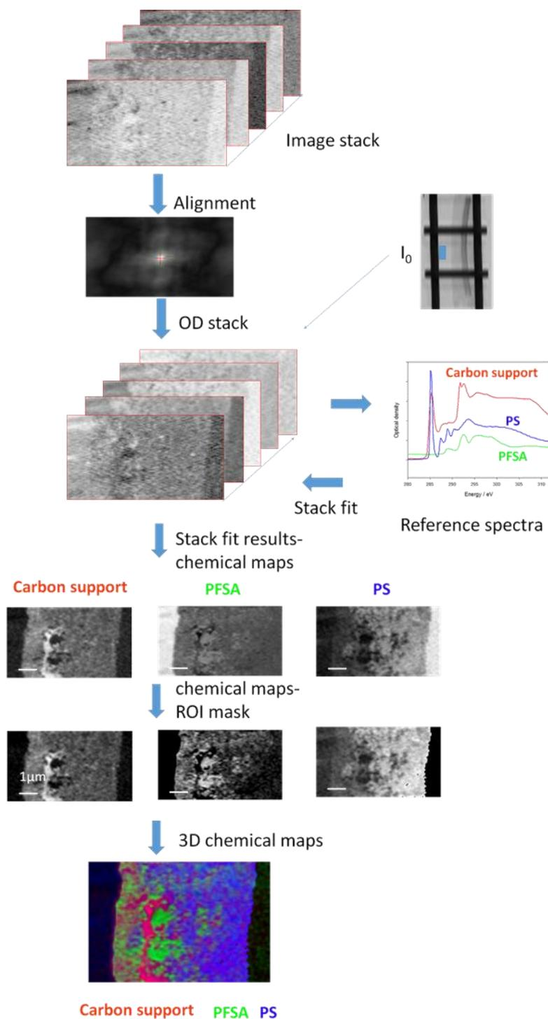
**Figure 3.4** Outline of processing of a STXM stack process of an MEA cathode sample. The image stack is measured in transmission mode by STXM; stack alignment in “Zimba” or “Jacobsen”; convert to OD stack; generate component spectra; stack fit using reference spectra; ROI mask; 3D chemical maps in color map
