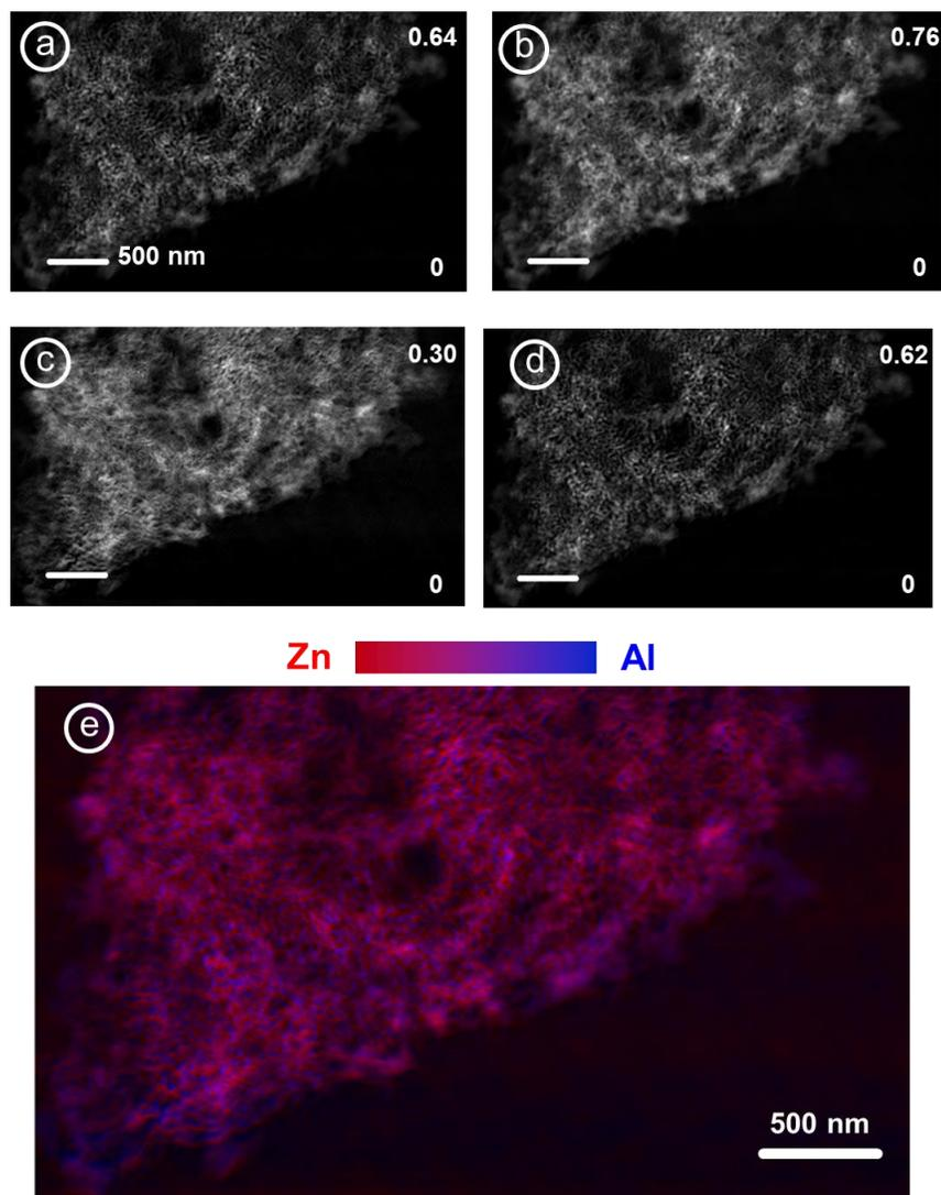
**Figure 7.5** Ptychography absorption images of ZnO/ $\text{Al}_2\text{O}_3$  aerogel (**sample B**) at (a) 1010 eV, (b) 1026.8 eV. (c) ZnO chemical map ( $\text{OD}(1026.8 \text{ eV}) - \text{OD}(1010 \text{ eV})$ ). (d) Derived  $\text{Al}_2\text{O}_3$  chemical map (see text). (e) 4D image color composite of the two component maps, ZnO in red,  $\text{Al}_2\text{O}_3$  in blue.
