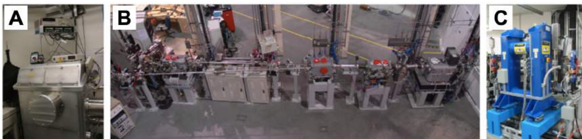
Figure 3.10 10ID SM beam line at the CLS: (A) STXM. (B) SM beamline. (C) Elliptically polarizing undulator (EPU) (Kaznatcheev et al., 2007). With permission from Elsevier.
