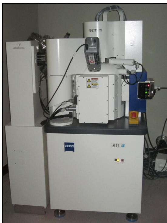
Figure 3.28 Zeiss NVision 40 dual FIB/SEM used for FIB modification of the CNT.
