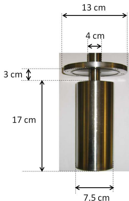
Figure 3.13 Cold finger designed and fabricated for the CLS STXM.
