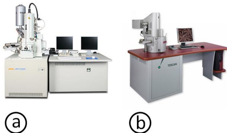
Figure 3.9 7000F JEOL (a) and Tescan Vega II (b) SEM used to preview the CNT samples prior to STXM measurements.
