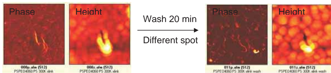
Figure 6.3: AFM height and phase mode images for a PS-PEO 40:60 film imaged before and after immersion in DDI water for 20 min.
