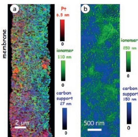
**Fig. 1:** (a) Color coded composite of Pt (red), carbon support (blue) and perfluorosulfonate ionomer (green) in anode of an automotive polymer electrolyte membrane fuel cell (PEM-FC) derived from a C 1s image sequence measured by STXM. (b) Color coded composite of carbon support (blue) and perfluorosulfonate ionomer (green) in the cathode of a PEM-FC measured by 2-energy F 1s spectro-ptychography [12]. Color intensity scales are quantitative thickness in nm.
