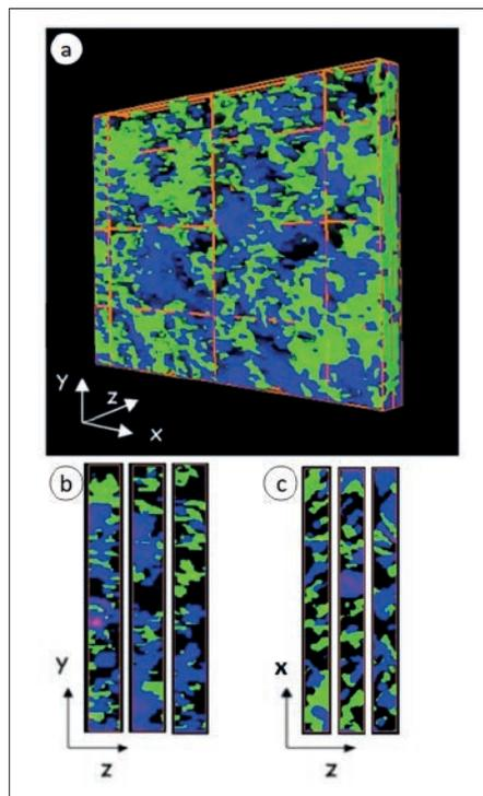
Fig. 2: (a) Perspective view of 3D chemical structure of a PEM-FC cathode derived from a 14 tilt angle, 2-energy (684, 694 eV) spectro-ptycho-tomography measurement on a microtomed sample. Carbon support is blue, ionomer is green. The slab has dimensions of  $4 \mu\text{m} \times 4 \mu\text{m} \times 250 \text{nm}$ . (b) cuts in the y-z plane from 3 x positions. (c) cuts in the x-z plane from 3 y positions [12].
