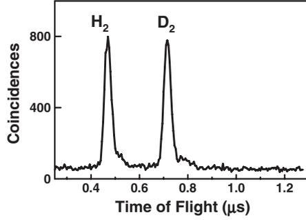
FIG. 2. TOF spectrum of the  $H_2$ - $D_2$  mixture obtained by (e, e + ion) at an energy loss of 20 eV and  $4^\circ$  scattering angle.
