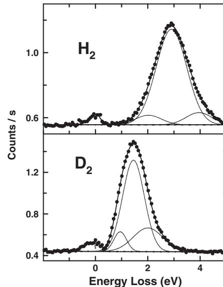
FIG. 1. Quasielastic electron energy loss spectra of H<sub>2</sub> and D<sub>2</sub>, showing fits of 3 Gaussian curves to the experimental data. The small peaks on the low energy side arise from incomplete subtraction of the quasielastic peaks due to background air in the spectrometer.
