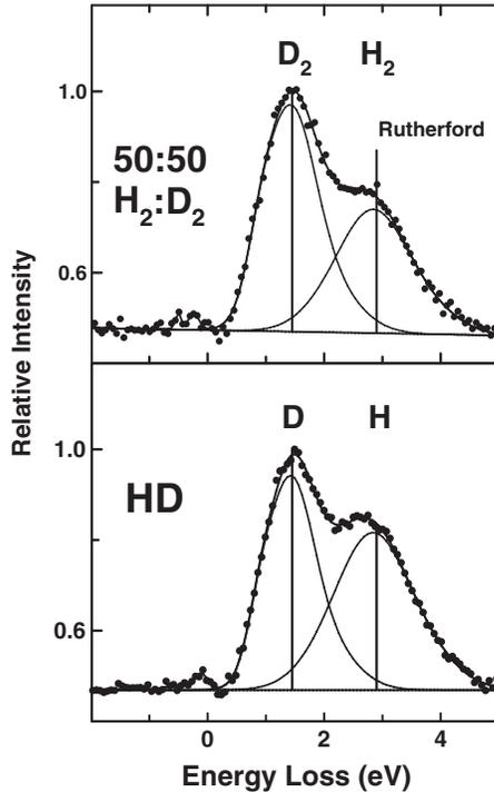
FIG. 3. Quasielastic electron energy loss spectra of the 50:50  $H_2$ - $D_2$  mixture and of HD. The fits of curves representing the individual H and D scattering peaks to the experimental data are shown. The vertical lines show the calculated recoil energies  $\hbar\omega_r = (\hbar q)^2/(2M_i)$  for  $i = H, D$ .
