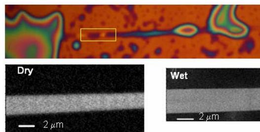
**Figure 2** (upper) Optical image and (lower) STXM OD images (at 288.2 eV) of dry and fully water saturated *N. clavipes* dragline silk fiber embedded in epoxy.
