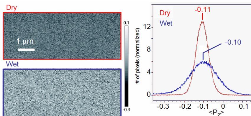
**Figure 3.** (left)  $\langle P_2 \rangle$  orientation maps of dry and wet fiber sections displayed on the same intensity scale. (right) Comparison of histograms of  $\langle P_2 \rangle$  values for the dry (blue) and wet (red) fibers.
