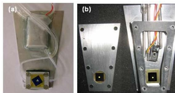
**Figure 1.** (a) First version of humid cell with the humidity sensor only connected to sample compartment via thin tubing. (b) Mark II humid cell with sensor, dry and humid He ports and thermocouple integrated into the sample region.
