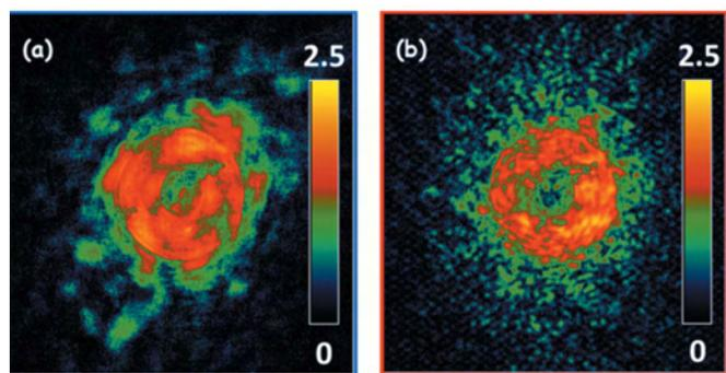
**Figure 5** Effect of spot size on diffraction images (DIs). (a) X-ray scattering signal from the BN sample using focused beam (diameter of 62 nm). (b) X-ray scattering signal from the same spot as in (a) using a defocused beam of diameter 1000 nm. Both DIs were recorded at 192 eV and LH polarization, and a sample-to-camera distance of 51.3 mm.
