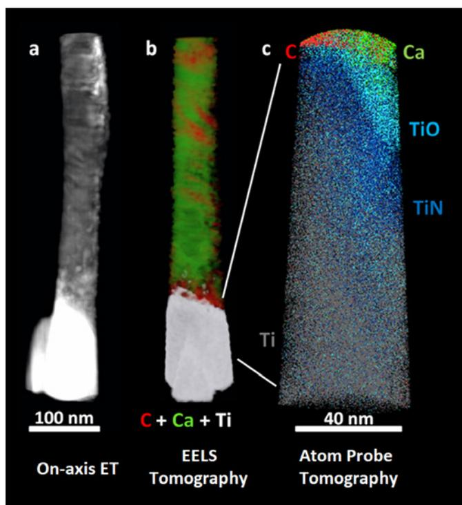
**Figure 2:** (a) On-axis ET, (b) electron energy loss tomography (EELS ET), (c) APT of the interface of human bone and a Ti dental implant. The TiO and TiN designations are related to detailed analysis of the O and N species from APT spectra [3]. (Adapted from [3]).
