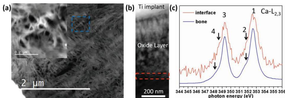
**Figure 4.** ELNES comparison of Ca- $L_{2,3}$  from bone and interface. HAADF-STEM images of a) mature bone and b) bone–implant interface, where the titanium oxide layer spans roughly 300 nm past the bright Ti substrate. c) Ca- $L_{2,3}$  edges of bone (in blue) and interface (in red) are extracted from the regions highlighted by the dashed squares in corresponding colors in panels (a) and (b). Four discernable peaks are indicated by arrows and their accurate positions are included in Table 1.
