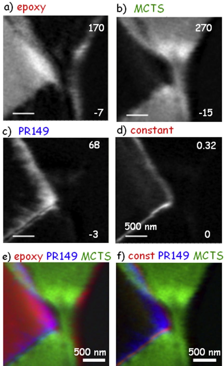
**Fig. 4.** Higher magnification maps and color coded composites for an uncoated NSTF whisker sample. The component maps for (a) epoxy, (b) MCTS, (c) PR149 and (d) constant were derived by a stack fit analysis of a C 1s image sequence. The numbers on the epoxy, MCTS, and PR149 images indicate the minimal and maximal thickness in nm, while that for the constant image indicates the minimal and maximal OD. (e) and (f) are color coded composites (rescaled) of the indicated components.
