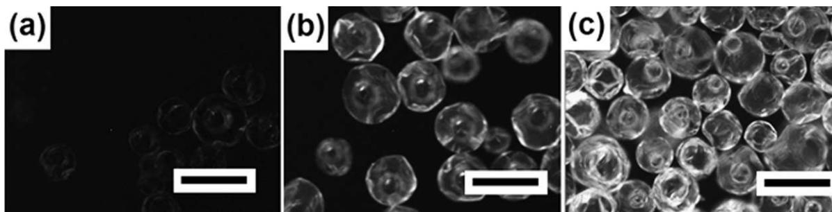
**FIGURE 5** Conventional fluorescence microscope images of polyurea microcapsules using an FITC filter set (a) native capsules; (b) (A70f/PAPMr)-modified capsules; and (c) (A70f/PAPMr)<sub>2</sub>-modified capsules. All scale bars denote 50  $\mu\text{m}$ .
