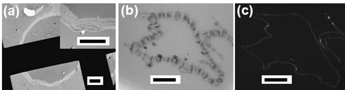
**FIGURE 6** Wall cross-section of a (A70/PAPMn)<sub>2</sub>-modified polyurea microcapsule. (a) A TEM micrograph showing a capsule cross-section (the insert in the upper right hand corner is the enlarged image of the boxed area). (b) An optical microscope image and (c) A fluorescence microscope image (greyscale). (b) And (c) were taken in the same sample area. Scale bars denote 10  $\mu\text{m}$ .
