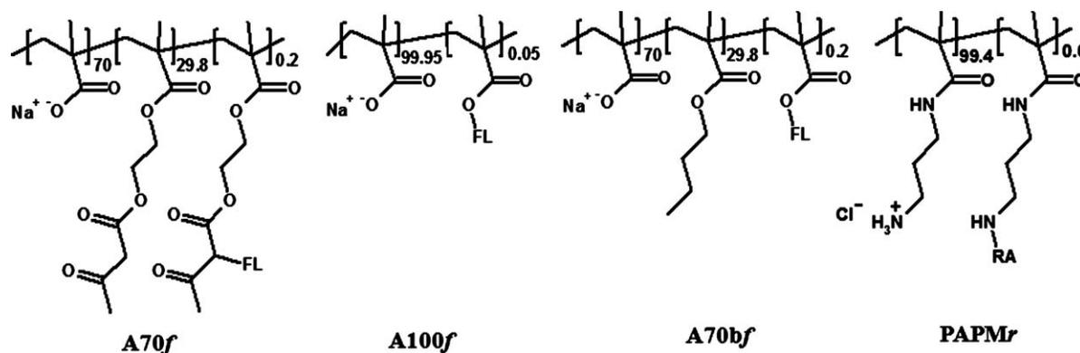
**SCHEME 1** Chemical structures of fluorescein-labeled poly(sodium methacrylate-*co*-2-(methacryloyloxy) ethyl acetoacetate) (A70f), fluorescein-labeled poly(methacrylic acid) (A100f), fluorescein-labeled poly(methacrylic acid-*co*-butyl methacrylate) (A70bf), and rhodamine-labeled poly(*N*-(3-aminopropyl) methacrylamide) (PAPMr). FL: fluorescein; RA: rhodamine.
