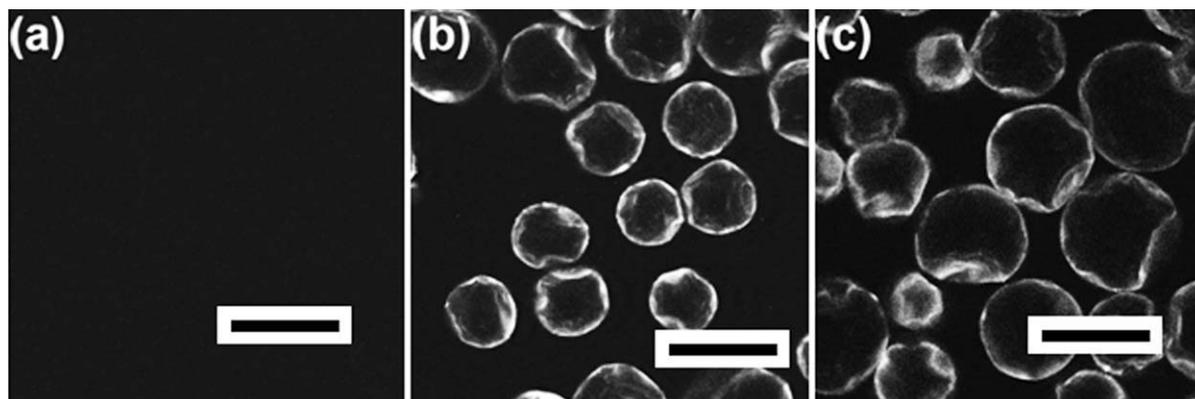
**FIGURE 3** Confocal microscopy images (greyscale) of PUMCs: (a) without modification; (b) modified by A70f; and (c) first modified by A70f and then treated with 2 M NaCl solution. All scale bars stand for 50  $\mu\text{m}$ .
