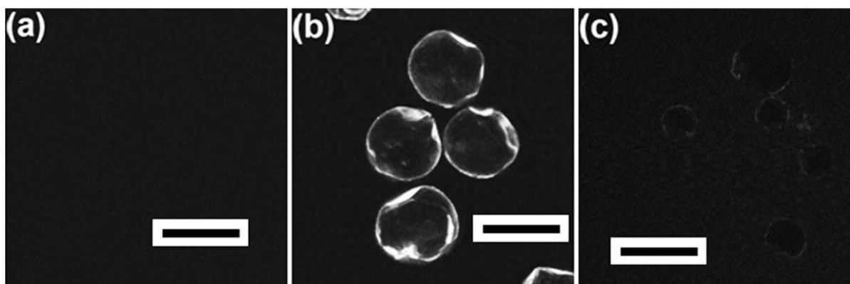
**FIGURE 2** Equatorial confocal fluorescent microscope images (greyscale) of polyurea microcapsules (a) without treatment, (b) after treatment with FITC, and (c) after treatment with A100f. All scale bars are 50  $\mu\text{m}$ .
