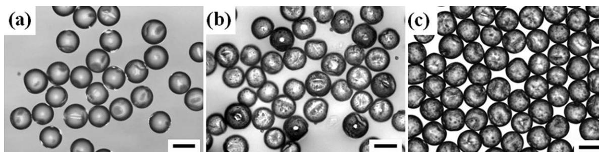
**FIGURE 9** Optical micrographs of narrowdisperse aromatic polyurea microcapsules made using the microfluidic device at room temperature with different reaction time: (a) 1 hour; (b) 2 days; and (c) 7 days. The scale bars are 100 µm.
