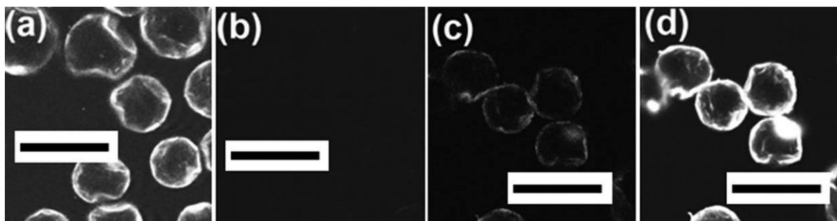
**FIGURE 4** Confocal images (greyscale) of A70f-coated polyurea microcapsules in: (a) FITC channel (b) rhodamine channel; and A70f/PAPMr bilayer polyurea microcapsules in (c) FITC channel and (d) rhodamine channel. All scale bars denote 50  $\mu\text{m}$ .
